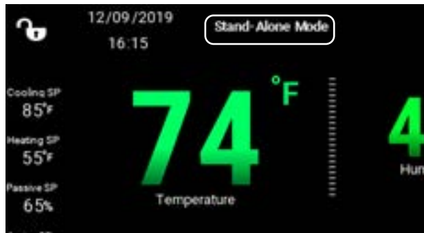
FIGURE 18 Unit Status Displayed on Main Screen
