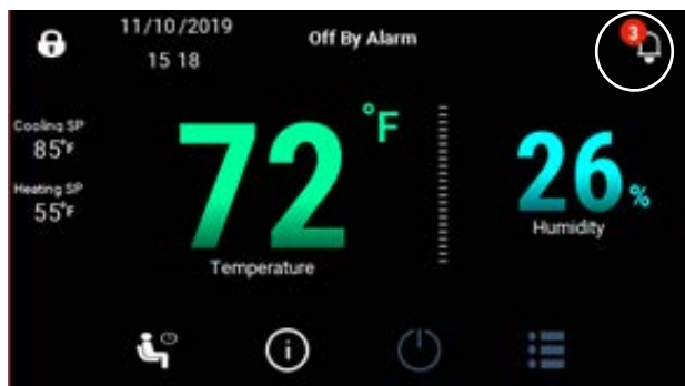
FIGURE 19 Active Alarms Displayed on Main Screen
