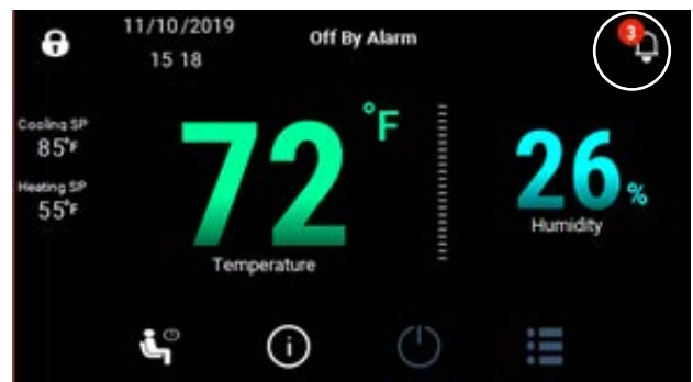
FIGURE 19 Active Alarms Displayed on Main Screen
