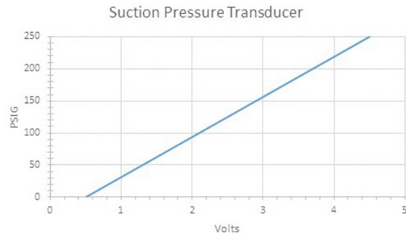
FIGURE 25 Voltage to Pressure: Suction Pressure Transducer
