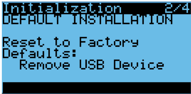
FIGURE 12 Restoring Factory Default Settings – Remove USB Device
