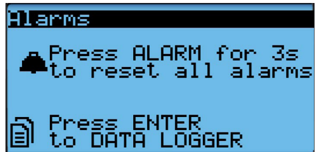
FIGURE 13 Clearing All Alarms
