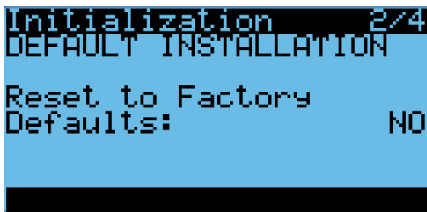
FIGURE 11 Restoring Factory Default Settings
