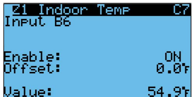
FIGURE 39 Enable/Disable Zone 1 Indoor Temperature Sensor
