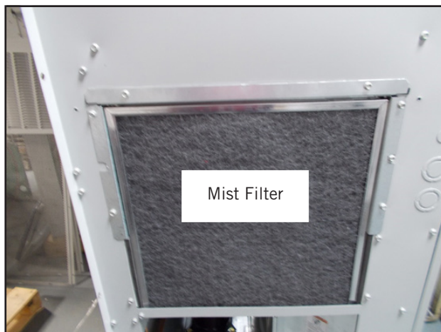
FIGURE 26 Install Mist Filters
