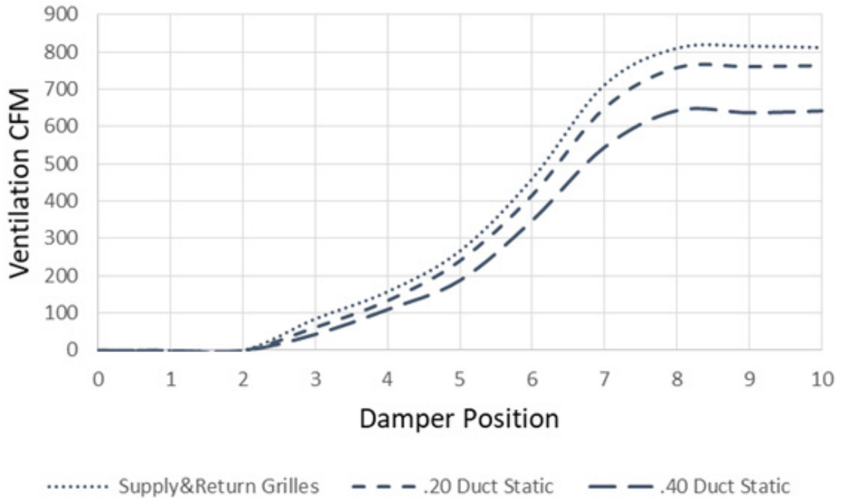
GRAPH 1 W3SAC CRV-V5 Ventilation Delivery
