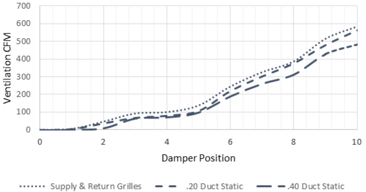
GRAPH 3 W30 Ventilation Delivery
