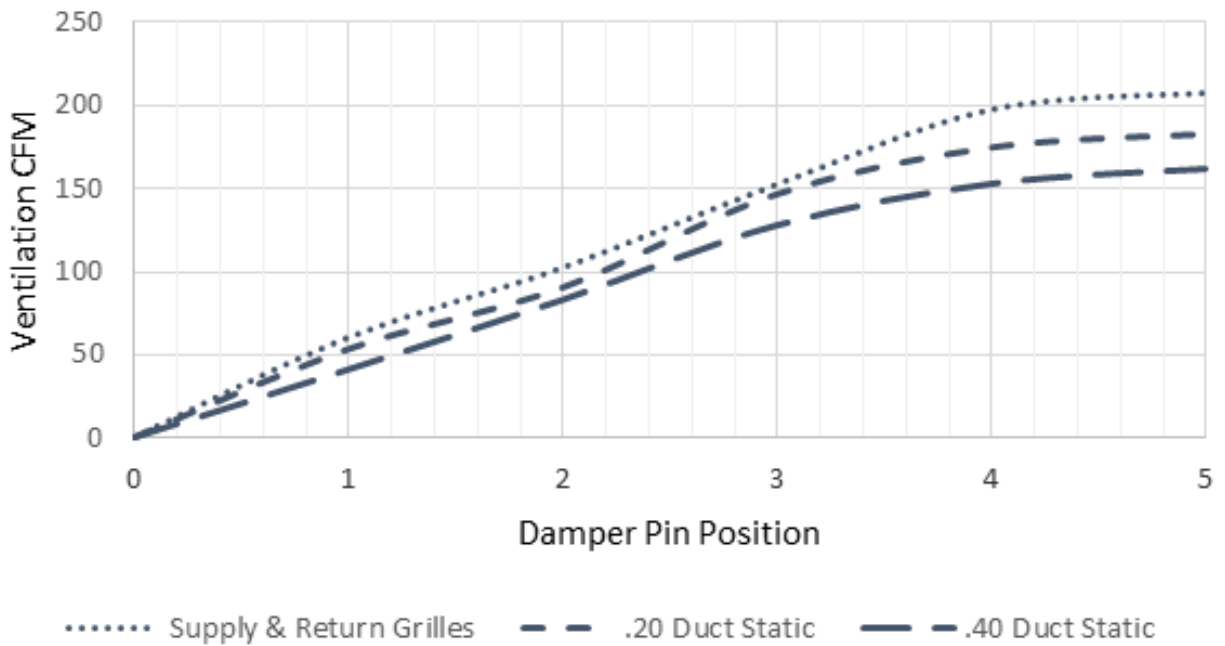
GRAPH 4 J36HY FAD-NE2, 3 W/O Exhaust Ventilation Delivery
