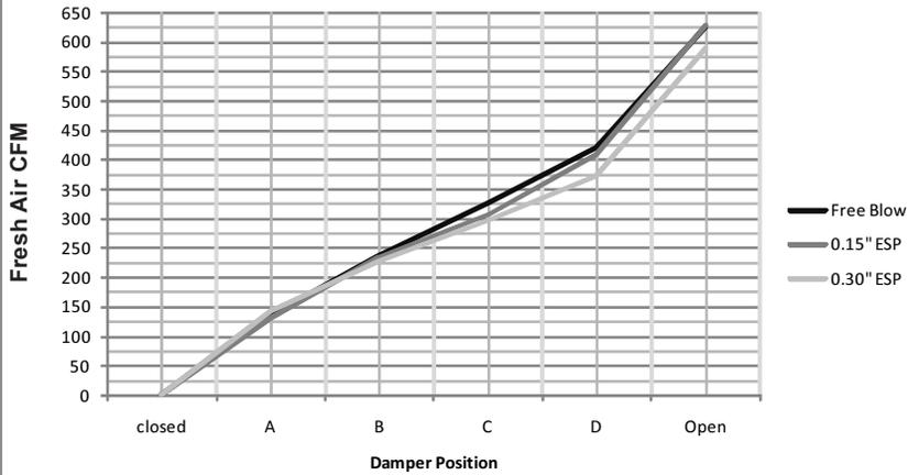
**W42-60G CRV Airflow Versus Position - Medium Speed**
