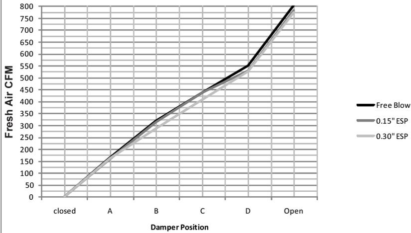
**W42-60G CRV Airflow Versus Position - High Speed**
