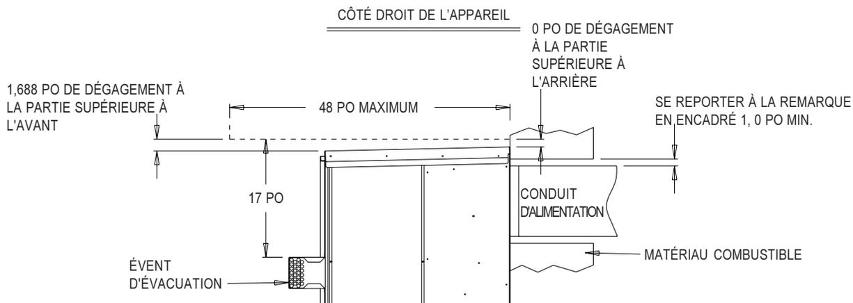
VUE EN COUPE LATÉRALE DU CONDUIT D'AIR D'ALIMENTATION DE L'APPAREIL FIXÉ AU MUR MONTRANT UN DÉGAGEMENT DE 1 PO PAR RAPPORT À TOUTES LES SURFACES COMBUSTIBLES.
