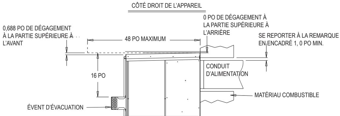
VUE EN COUPE LATÉRALE DU CONDUIT D'AIR D'ALIMENTATION DE L'APPAREIL FIXÉ AU MUR MONTRANT UN DÉGAGEMENT DE 1 PO PAR RAPPORT À TOUTES LES SURFACES COMBUSTIBLES.
